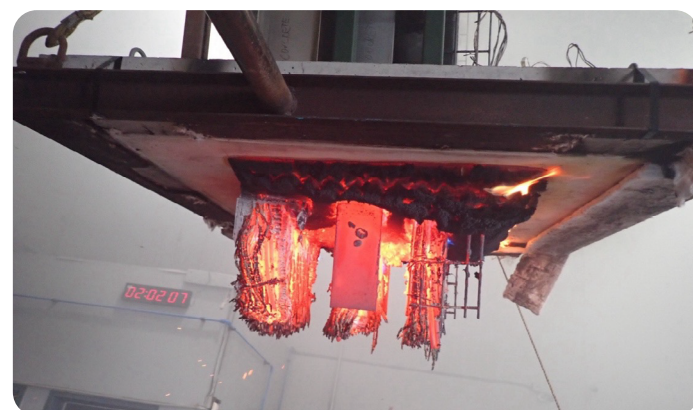
Firestop Block Installation Upon Completion of Fire Endurance Testing (C-AJ-4121)
