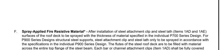
with spray applied fire resistive material to the minimum thickness of material required on the flanges of the steel beam.
