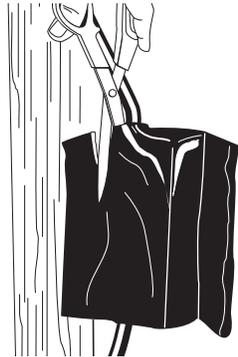
If wall membrane is in place, pack putty into gaps between box and wallboard slightly overlapping inner wallboard surface. If membrane is to be installed after pad installation, overlap front edge of box so that putty will be compressed around edges of box as wallboard is installed. Cut slits in pad to fit around conduits or cables.
