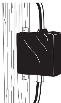
Align pad to the side of box partially overlapping the stud and adhere. Work to opposite side of the box to the edges.
