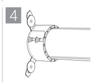
Fasten all collar anchor tabs to mounting surface using approved fasteners.
