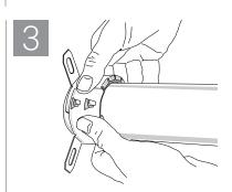
Press slots down and back (towards mounting surface) over hooks and lock into the closed position.
