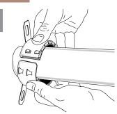
Flex collar open and wrap around pipe; anchor tabs to be facing mounting surface.
