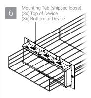
Insert provided mounting tabs into slots on top and bottom of device through clear nameplates as shown. Align holes and fasten mounting tabs to slim mounting frames using the screws provided. Fill any unoccupied
