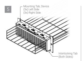
Attach top half of device to bottom half by inserting the interlocking tabs into the rectangular slots on each side of device. Secure device halves together using screws from Step 1. Align holes and fasten mounting tabs of device to slim mounting frames using the screws provided.
