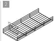
Fasten Slim Mounting Frame, Left to wall so that it covers the opening in the wall. Orient frame with the double layer stack of wrap strip and both rivets towards the top. See table on second page for fastener types.
