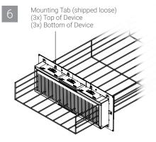
Insert provided mounting tabs into slots on top and bottom of device through clear nameplates as shown. Align holes and fasten mounting tabs to slim mounting frames using the screws provided. Fill any unoccupied holes using the screws provided.
