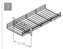
Fasten Slim Mounting Frame, Right to wall so that it covers the opening in the wall, placing the ends over the Slim Mounting Frame, Left. Orient frame with the double layer stack of wrap strip and both rivets towards the top. Verify horizontal CL hole to CL hole dimension shown. See table on second page for fastener types.
