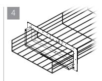
Tightly abut bottom half of tray device against underside of cable tray and face of slim mounting frames. Align holes and fasten mounting tabs of device to slim mounting frames using the screws provided.
