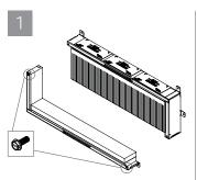
Remove corner screws and separate device into two halves.
