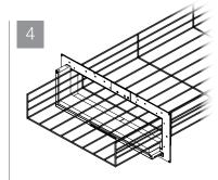
Tightly abut bottom half of tray device against underside of cable tray and face of slim mounting frames. Align holes and fasten mounting tabs of device to slim mounting frames using the screws provided.
