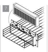
Re-insert intumescent foam strips, foam blocks, and rubber gasket assembly into device as shown.
