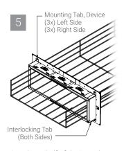
Attach top half of device to bottom half by inserting the interlocking tabs into the rectangular slots on each side of device. Secure device halves together using screws from Step 1. Align holes and fasten mounting tabs of device to slim mounting frames using the screws provided.
