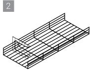
Fasten Slim Mounting Frame, Left to wall so that it covers the opening in the wall. Orient frame with the double layer stack of wrap strip and both rivets towards the top. See table on second page for fastener types.
