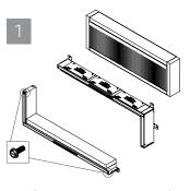
Remove corner screws and separate device into two halves. Remove intumescent foam strips. foam blocks, and rubber gasket assembly from top half of device.
