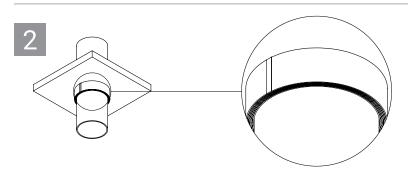
Continuously wrap min. six (6) layers of intumescent wrap strip around the pipe. Wrap strip to be installed flush with the bottom surface of the floor or both sides of the wall. Use tape at the wrap strip seam to temporarily hold the wrap strip in place.
