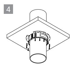
Fasten collar flanges to the bottom of the floor or both sides of the wall as required in the UL System
