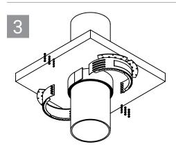
Position collar halves around the wrap strip with the flanges facing towards the bottom of the floor or side of the wall on both sides. Insert threaded bolts through slots in collar shells, and secure together using the provided washers and nuts. Ensure that collar flange is tight to the bottom surface of the floor or both wall surfaces.
