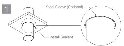
Install SpecSeal® Sealant as required in the UL system
