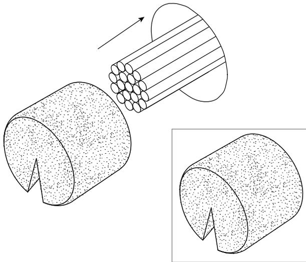
When cables are present, slit plug to accommodate single or grouped cables.
