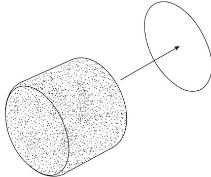
Insert plug into opening/sleeve on both sides of wall with rounded face positioned outward. Face of plug to be flush with wall surface.
