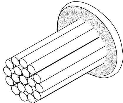
Cables to be centered within plug using slit opening. Rounded face of plug positioned outward and flush with wall surface on both sides of wall.
