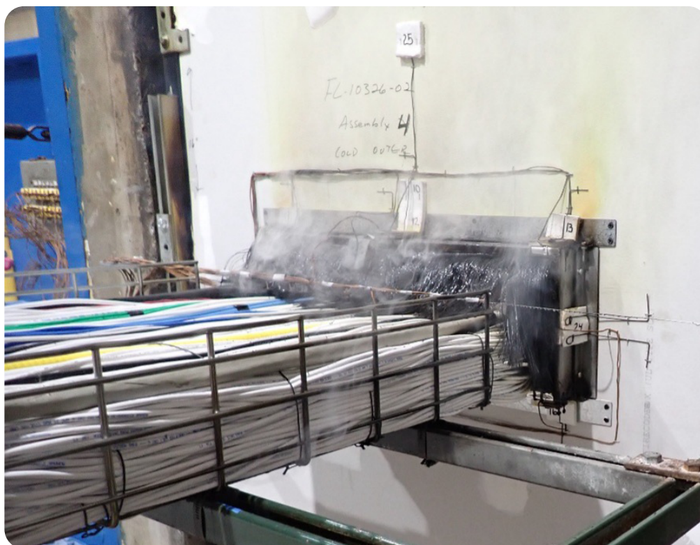
EZ Path® ULTRA During Fire Endurance Testing (W-L-4116)
