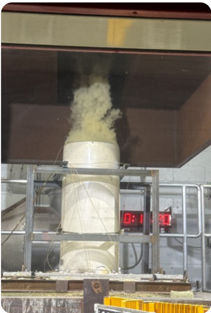
EXC Firestop Collar During Fire Endurance Testing (C-AJ-21008)
