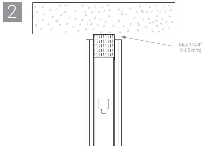
2 Max 1-3/4" (44.5 mm) wide joint between gypsum layer(s) and bottom surface of floor/deck.
