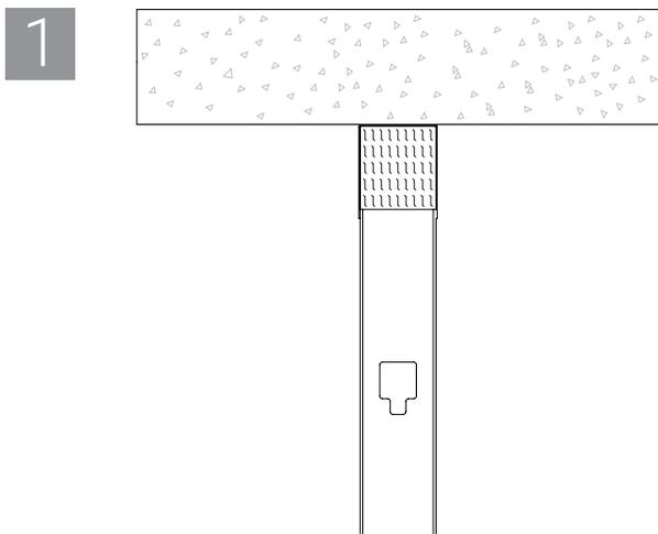
1 Mineral wool block compressed into ceiling runner and secured in place using cup head weld pins. See UL System for more detail
