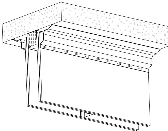
Profile fastened to wall surface using nom. 1/2" (13mm) steel staples spaced nom. 8" (203mm) OC. See UL System for more detail.
