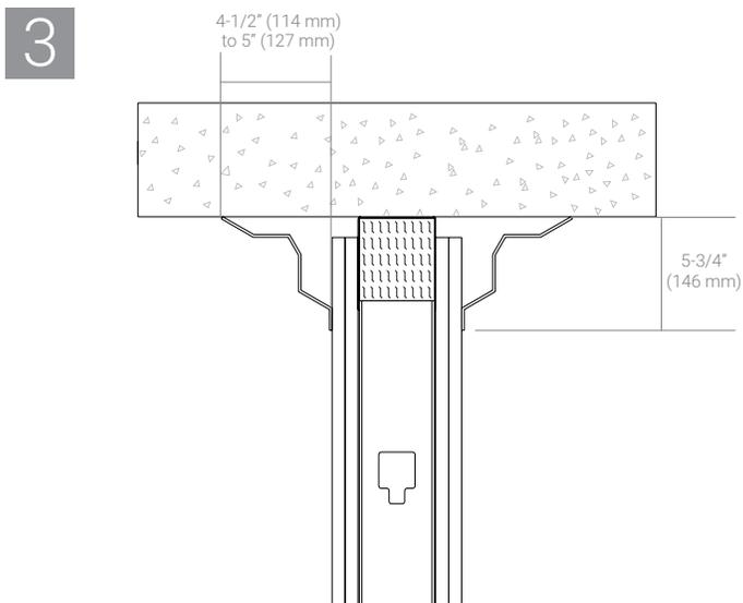
3 Place SFJP80 profile over joint on both sides of wall. Leg of Joint profile offset nom. 5-3/4" (146mm) from underside of floor/deck. Opposing leg offset from face of steel ceiling runner 4-1/2" (114mm) for 1Hr and 5" (127mm) for 2 Hr configurations. See UL System for more detail.
