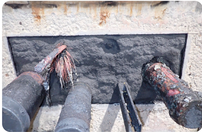
Exposed Side of Firestop Blocks Following Fire Endurance and Hose Stream Test (C-AJ-8360)
