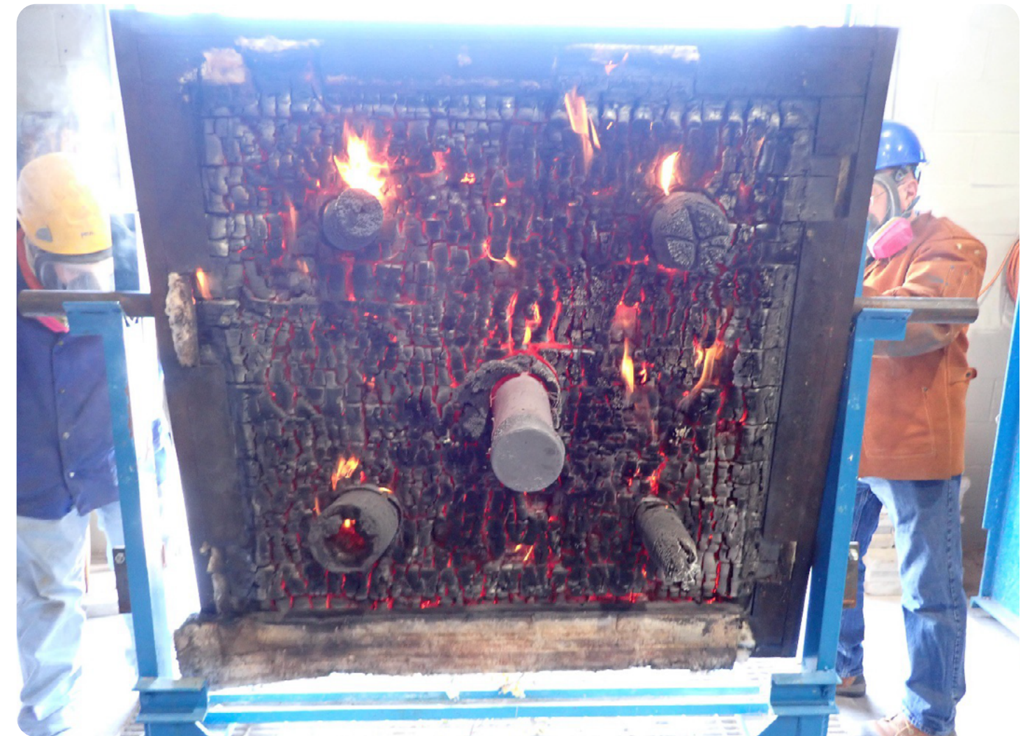
Intumescent Sleeves Following Fire Test in CLT Floor Assembly (F-G-1002, F-G-2004 and F-G-5003)
