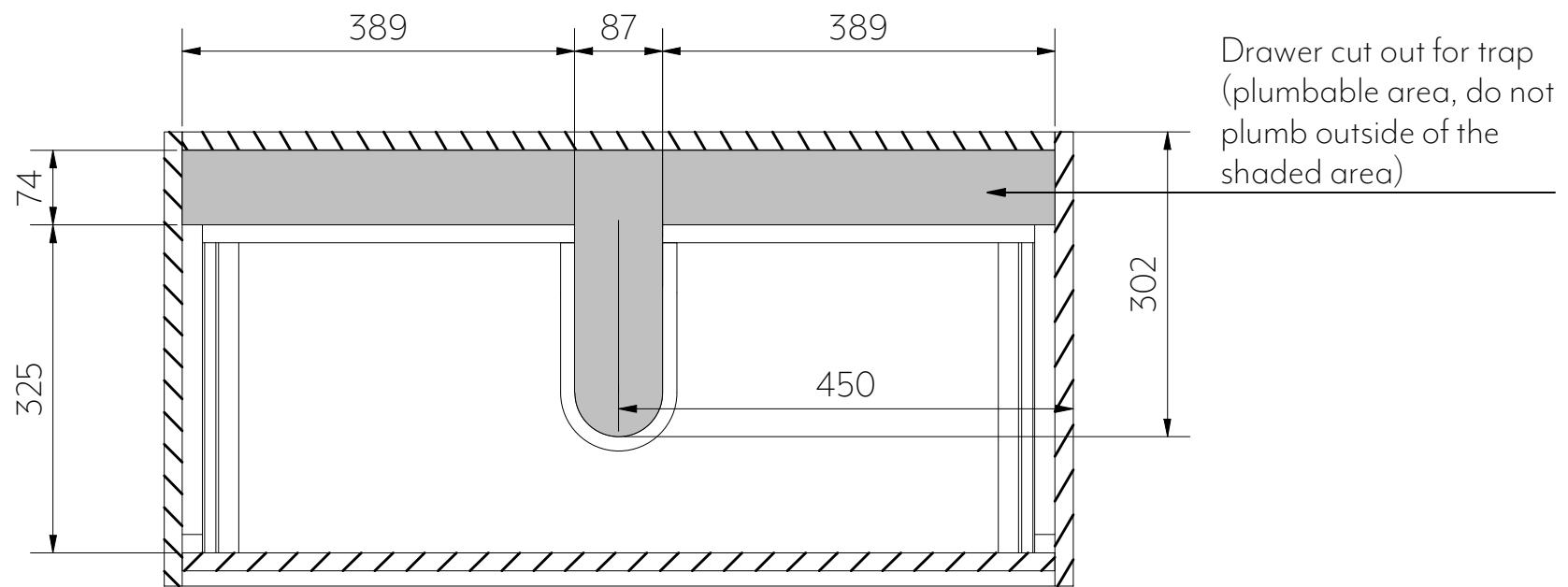
Cut out drawer must align with plumbing.
