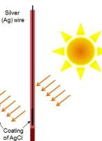
Ambient light, especially the daylight, reacts continuously with AgCl and reduces traces of silver ion to silver metal. This reduces the lifetime of the probe.
