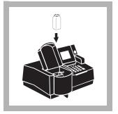
**12.** Place the prepared sample in the cell holder. Close the light shield. Results in mg/L SiO<sub>2</sub> (or chosen units) will be displayed.
