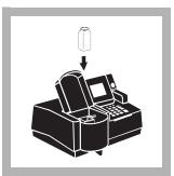
**10.** When the timer beeps, place the blank in the cell holder. Close the light shield.
