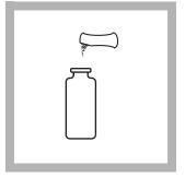
**8.** When the timer beeps, add the contents of one Amino Acid F Reagent Powder Pillow to one of the sample cells. Swirl to mix. This is the prepared sample.
