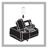
**8.** Place the prepared sample into the cell holder. Close the light shield. The result in g/L Nickel (or chosen units) will be displayed.
