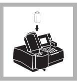
**6.** Place the blank into the cell holder. Close the light shield.
