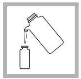
**3.** Fill a sample cell with 10 mL of deionized water (the blank).
