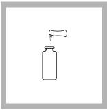
**5.** Add the contents of one Potassium 1 Reagent Powder Pillow to the sample (the prepared sample). Stopper and shake to dissolve.
