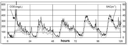
Figure 1 – Comparison of SAC and COD in the influent of a municipal wastewater treatment plant
