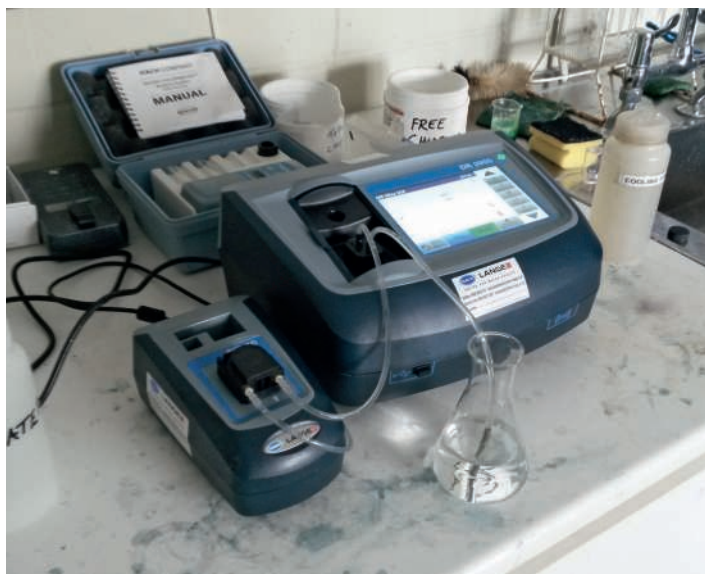
DR 3900 spectrophotometer with automated sipper cell module
