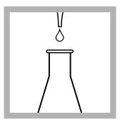
**12.** Add 5.25 N Sulfuric Acid Standard Solution, 1 drop at a time until the color changes from pure blue to purple and then to red.
