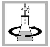
**17.** Put the flask under the buret. Swirl the flask. Add titrant until the color changes from red to pure blue.
