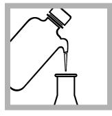
**5.** If the sample volume is less than 50 mL, dilute to approximately 50 mL with deionized water.
