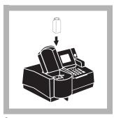
**9.** When the timer beeps, place the blank into the cell holder. Close the light shield.
