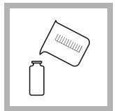
**4.** Fill another glass-stoppered sample cell to the 25-mL mark with deionized water (the blank).
