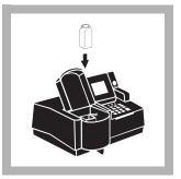
**11.** Place the prepared sample into the cell holder. Close the light shield. Result in mg/L ammonia as nitrogen (NH<sub>3</sub>–N) (or chosen units) will be displayed.
