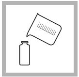
**3.** Fill a glass-stoppered sample cell to the 25-mL mark with sample.
