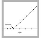
**13.** Draw the two best intersecting lines through the plotted points as shown above.
