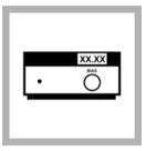
7. Note the LED reading on the Amperometric Titrator. It should read  $0.00 \pm 0.05$ . **DO NOT** adjust the bias control.
