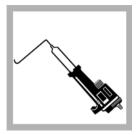
1. Install the Standard lodine Titrant Cartridge, 0.028 N. Flush the Digital Titrator delivery tube by turning the delivery knob to eject a few drops of titrant. Reset the counter to zero and wipe the tip.
