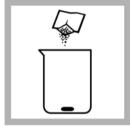
6. Add the contents of one Potassium Iodide Reagent Power Pillow to the beaker and allow the powder to dissolve.
