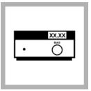
**11.** After the end point of the titration (nominal 160 digits), record the increasing LED readings along with the corresponding digits displayed on the Digital Titrator counter.
