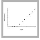
**13.** Use a linear graph paper to plot the recorded readings from the Amperometric Titrator on the vertical axis and the corresponding Digital Titrator digits on the horizontal axis.
