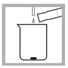
4. Add 1 mL of pH 4 Acetate Buffer Solution to the beaker. Then add 200 mL of the sample to the beaker.
