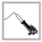
1. Flush the Digital Titrator delivery tube by turning the delivery knob to eject a few drops of titrant. Reset the counter to zero and wipe the tip.
