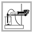
5. Place the beaker on the TitraStir stand and immerse the tips of both the probe and the delivery tube in the solution. The probe's platinum wires must be submerged. Turn on the stirring motor.
