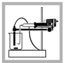
8. Using the Digital Titrator delivery knob, dispense Standard Iodine Titrant Solution in five to ten digit increments while noting the reading.
