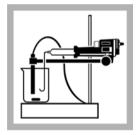
8. Using the Digital Titrator delivery knob, dispense 100 digits of Standard lodine Titrant Solution and note the reading.
