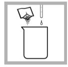
5. Add 1 mL of pH 4 Acetate Buffer Solution and the contents of one Potassium Iodide Powder Pillow.
