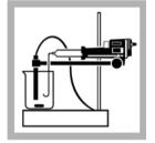
6. Place the beaker on the TitraStir stand and immerse the tips of both the probe and the delivery tube in the solution. The probe's platinum wires must be submerged. Turn on the stirring motor.
