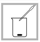
**4.** Use a Class A pipet to transfer 1.00 mL of 0.00564 N Sodium Thiosulfate Solution to the beaker. Swirl to mix.
