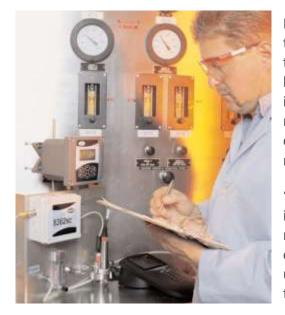
Dooley also noted that drift has been minimal during the several months the system has been in place, and that the design of the new flow cell makes it easy for his laboratory technicians to access the electrode and immerse it in buffer solution when calibration is required. Instrument set-up and calibration proved easy—even intuitive—simply by following the display menu.
