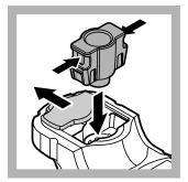
**3.** After startup, install the vial adapter. Push in the tabs on the sides of the vial adapter as shown.
