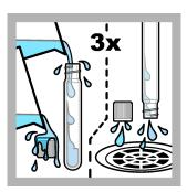
**6.** Rinse the sample vial and cap three times with the sample.
