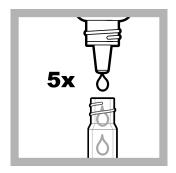
**8.** Add **5** drops of Fluorescence Free Chlorine **Reagent 2**. Hold the bottle vertically.
