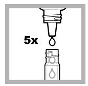
7. Add 5 drops of Fluorescence Free Chlorine Reagent 1. Hold the bottle vertically.
