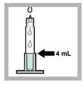
9. Put the sample vial in the sample vial holder. Add the sample to the top of the sample vial holder (4 mL). If more than 4 mL of sample is added, there is a very small effect on the result.
