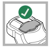
**2.** Keep the sample port cover closed during startup.
