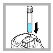
**12.** Put the sample vial in the vial adapter.
