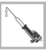
2. Hold the Digital Titrator vertically with the cartridge tip up. Turn the delivery knob to eject air and a few drops of titrant. Reset the counter to zero and clean the tip.
