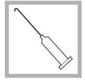
**1.** Insert a clean delivery tube into the Mercuric Nitrate Titration Cartridge. Attach the cartridge to the Digital Titrator.
