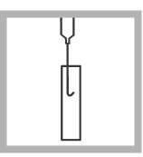
6. Put the delivery tube point fully into the solution and swirl the flask. Turn the knob on the Digital Titrator to add titrant to the solution. Continue to swirl the flask and add titrant until the color changes from yellow to light pink. Record the number of digits on the counter.
