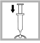
**3.** Use the 3-mL (3-cc) syringe to collect a 2.0-mL (2-cc) water sample. Add the sample to the plastic vial.
