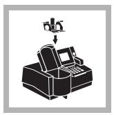
12. Insert the Test 'N Tube Adapter into the sample cell module by sliding it under the thumb screw and into the alignment grooves. Fasten with the thumb screw.
