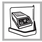
**1.** Turn on the COD Reactor. Heat to 103–106 °C (best temperature is 105 °C). Place the plastic shield in front of the reactor.
