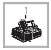
13. When the timer beeps, clean the outside of the TN Reagent C Vial containing the reagent blank. Place the vial in the adapter and close the light shield.
