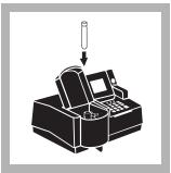
**16.** Place the prepared sample into the cell holder and close the light shield. The result in mg/L total nitrogen will be displayed.
