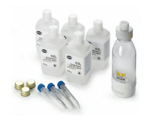
Hach has measured the solubility of  $CO_2$  in the final calibration solution at different temperatures and computed correction tables for various analyzer settings (patent pending). The calibration tables will be delivered in the starter kit and will tell the user which number to enter in their instrument during calibration or which value they should read on their display during a verification, depending on analyzer settings.
