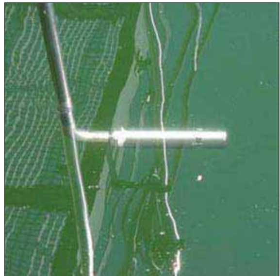
Figure 3 – The Hach UVAS sc Sensor measures SAC without sample collection or reagents
