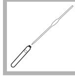
7. Prepare a blank by repeating steps 3 to 6, substituting 2.00 mL (0.2 mL for the 0 to 15,000 mg/L range) deionized water for the sample. Place the blank in the COD Reactor.
