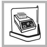
**9.** Turn the reactor off. Wait about 20 minutes for the vials to cool to 120 °C or less.
