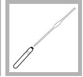
**4.** Hold the vial at a 45-degree angle. Pipet 2.00 mL (0.2 mL for the 0 to 15,000 mg/L range) of sample into the vial.
