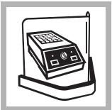
**2.** Turn on the COD Reactor. Preheat to 150 °C. Place the plastic shield in front of the reactor.
