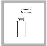
**4.** Add the contents of one Copper Masking Reagent Powder Pillow to one of the sample cells (the blank). Swirl to dissolve.
