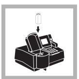
10. Place the prepared sample into the cell holder. Close the light shield. Results in  $\mu$ g/L copper (or chosen units) will be displayed.
