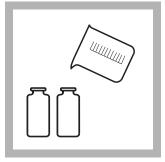
**3.** Fill two sample cells with 10 mL of sample.
