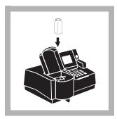
**13.** Place the blank into the cell holder. Close the light shield.
