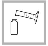
**3.** Using a graduated cylinder, fill a sample cell with 10 mL of sample.
