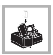
**9.** Place the prepared sample into the cell holder. Close the light shield. Results in mg/L F-(or chosen units) will be displayed.
