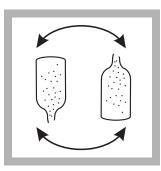
**5.** Quickly invert the ampuls several times to mix. Wipe off any liquid or fingerprints.
