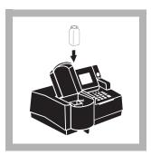
**7.** When the timer beeps, place the blank into the cell holder. Close the light shield.
