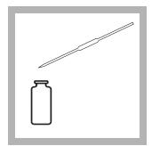
**4.** Pipet 10.0 mL of deionized water into a second dry sample cell (the blank).
