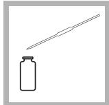
**3.** Pipet 10.0 mL of sample into a dry sample cell (the prepared sample).
