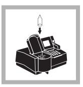
**8.** When the timer beeps, place the blank into the cell holder. Close the light shield.
