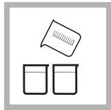
**3.** Collect at least 40 mL of sample in a 50-mL beaker. Pour at least 40 mL of deionized water into a second beaker.
