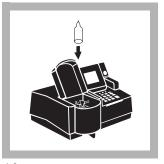
**10.** Place the AccuVac Ampul containing the sample into the instrument. Close the light shield. Results in mg/L F-(or chosen units) will be displayed.
