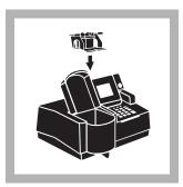
7. Insert the AccuVac Ampul Adapter into the sample cell module by sliding it under the thumb screw and into the alignment grooves. Fasten with the thumb screw.
