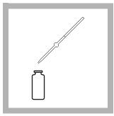
**5.** Use a pipet filler to pipet 2.0 mL of SPADNS Reagent into each cell. Swirl to mix.
