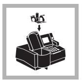
**4.** Insert the Test 'N Tube Adapter into the sample cell module by sliding it under the thumb screw and into the alignment grooves. Fasten with the thumb screw.
