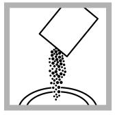
3. Add the contents of one PhosVer 3 Phosphate Reagent Powder Pillow to the sample cell. A blue color will show if phosphorus is in the sample.
