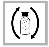
**3.** Quickly invert the AccuVac Ampul several times to mix.
