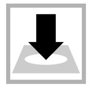
7. Insert the blank into the cell holder. Point the diamond mark on the sample cell toward the keypad.
