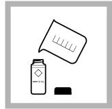
2. Prepare the sample: Rinse a sample cell and cap three times with sample. Fill the sample cell to the 10-mL mark with sample.
