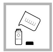
**6. Prepare the blank:** Rinse a sample cell and cap three times with sample. Fill the sample cell to the 10-mL mark with sample. Close the sample cell.
