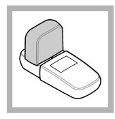
**9.** Install the instrument cap over the cell holder.
