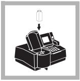
7. Insert a 1-cm cell adapter into the cell compartment. Place the blank into the 1-cm adapter with the clear windows aligned with the light beam. Close the light shield.
