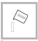
**9.** Discard the blank water from the cell and rinse the cell several times with filtered sample. After rinsing, fill the cell with filtered sample. Wipe the cell walls to remove fingerprints.
