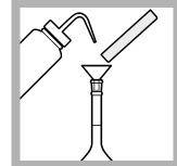
**4.** Rinse the pan and funnel several times with n-hexane. Add the rinse to the volumetric flask.
