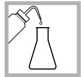
**12.** Rinse the Erlenmeyer flask with 5 mL of n-hexane. Add the n-hexane to the funnel. Set the vacuum to on and then to off.
