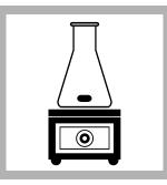
**6.** Add a stir bar to the flask. Stir for 5 minutes.
