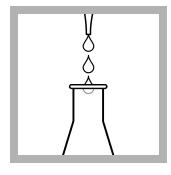
**7.** Remove the amount calculated in step 6 from the volumetric flask and add it to a 125-mL Erlenmeyer flask.
