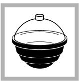
**2.** Remove the dish from the oven. Let the dish temperature decrease to room temperature in a desiccator.
