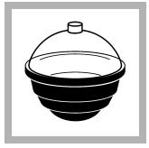
**31.** When the dish is dry, put the dish in a desiccator for 30 minutes.
