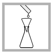
**3.** Pour the mixture into a 125-mL Erlenmeyer flask. Rinse the pan and funnel several times with n-hexane. Add the mixture to the flask.
