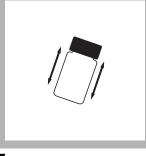
7. Cap the cell tightly and invert it several times. The solution will become hot. Cool to room temperature before proceeding.
