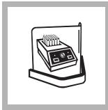
**17.** Place the vials in the COD Reactor that is preheated to 150 °C. Digest for 1 hour.
