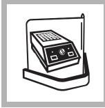
**3.** Turn on the COD Reactor and heat to 150 °C while preparing the sample and blank.
