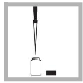
**5.** Using a TenSette Pipet or a pipet and safety bulb, pipet 9.0 mL of homogenized sample into an empty glass mixing cell. If the sample COD exceeds 1000 mg/L, dilute the sample as described in *Table 1*.
