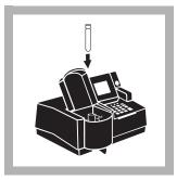
**24.** Place the sample vial in the adapter. Close the light shield. Results in mg/L COD (or chosen units) will be displayed.
