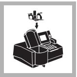
**20.** Insert the COD Vial Adapter into the sample cell module by sliding it under the thumb screw and into the alignment grooves. Fasten with the thumb screw.
