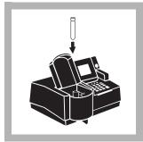
**21.** Place the blank into the sample cell compartment. Close the light shield.
