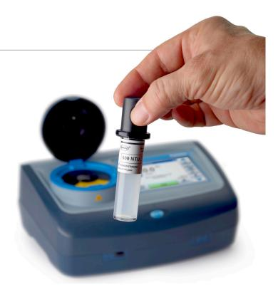
Did you know that both EPA and ISO regulations for all turbidity measurements require a calibration using primary standards? Secondary standards are convenient verification tools, but must also be calibrated against a primary standard.
