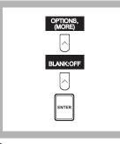
**3.** Account for the Molybdate 3 reagent blank by pressing the soft keys under *OPTIONS*, *(MORE)*, and then *BLANK:OFF*. Enter the reagent blank value found on the Molybdate 3 Reagent label and press **ENTER** until the read screen appears.
