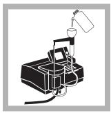
**20.** Flush the Flow-Thru or Sipper Cell with at least 50 mL of deionized water immediately after use.
