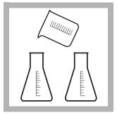
**5.** Fill two clean 250-mL Erlenmeyer flasks to overflowing with the sample to be tested.
