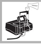
**15.** When the timer beeps, pour the contents of one flask into the Flow-Thru Cell or draw the contents into the Sipper Cell.
