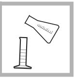
**8.** Fill this rinsed cylinder to the 50-mL mark with sample from the same flask, discarding any remaining sample in the flask.
