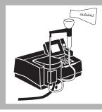
**18.** Wait 15 seconds (but no more than 5 minutes) for color formation. Transfer the contents of the second flask into the Flow-Thru Cell or draw them into the Sipper Cell.
