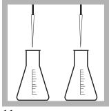
**11.** Using a TenSette Pipet, add 1.0 mL of Molybdate 3 Reagent to each flask. Swirl to mix.
