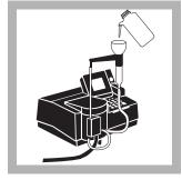
**4.** Insert the Flow Cell or Sipper Module and flush with 50 mL of low-silica deionized water.
