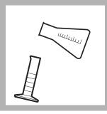
**7.** Repeat the rinsing of the cylinder three times from the same sample flask, discarding each rinse.
