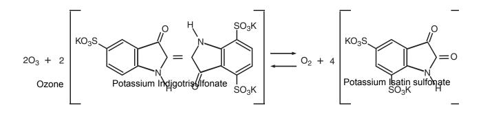
Figure 1 Chemical reaction for ozone determination, indigo method
