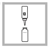
7. Add 2 drops of Sulfite Reagent B (HPT 430 B). Swirl to mix.
