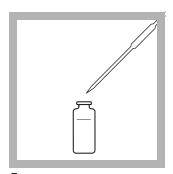
5. Pipet 10 mL of sample into a second sample cell.
