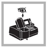
**3.** Place the DR/4000 1-inch Cell Adapter into the sample cell module by sliding it under the thumb screw and into the alignment grooves. Fasten with the thumb screw.
