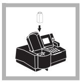
12. Place the prepared sample into the cell holder. Close the light shield. Results in mg/L Sulfite (or chosen units) will be displayed.
