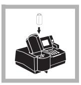
**10.** Place the blank cell into the cell holder. Close the light shield.
