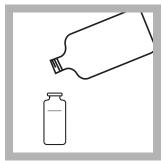
**4.** Fill a clean sample cell with 10 mL of deionized water. Cap the cell. This is the blank.
