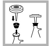
**4.** Assemble the filter holder/flask assembly using a clean filter flask.
