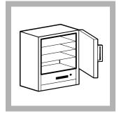
**1.** Put a clean evaporating dish in a drying oven at 180 °C (356 °F) for 1 hour.
