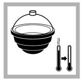
**16.** Remove the dish from the oven. Let the dish temperature decrease to room temperature in a desiccator.
