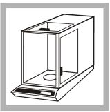
**12.** Use an analytical balance to weigh the dish to the nearest 0.1 mg (0.0001 g). Record this mg value as B.
