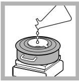
**14.** Pour the 100-mL filtrate sample from the filter flask into the evaporating dish. Dry for 4 hours. Examine the reservoir of the water bath at regular intervals. Add more water if necessary.
