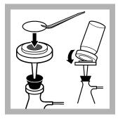
**5.** Use tweezers to put a 47-mm filter disc in the filter holder. Put the filter holder assembly in the filtering flask.
