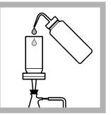
**6.** Connect vacuum to the filter holder/flask assembly and wash the filter with three separate 20-mL volumes of deionized water.
