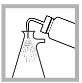
**3.** Remove all of the residue from the flask with a dilute solution of ammonium hydroxide. Rinse with deionized water.
