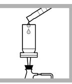
**10.** Use a clean 100-mL graduated cylinder to pour 100 mL (or more) of a well-mixed, representative water sample into the filter holder.
