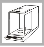
**17.** Use an analytical balance to weigh the dish to the nearest 0.1 mg (0.0001 g). Record this mg value as A. Do steps 15-16 again, until the difference between two successive sample weighings is less than 4% or 0.5 mg, whichever is less. If applicable, use the solid residue directly in method 8277 to determine Volatile Dissolved Solids.
