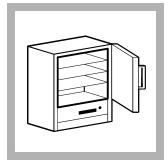
**15.** Put the evaporating dish in a drying oven at 180 °C (356 °F) for 1 hour.
