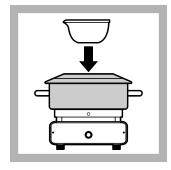
**13.** Put the steam bath on the hot plate. Add water to the steam bath. Put the evaporating dish in the steam bath.
