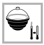
2. Remove the dish from the oven. Let the dish temperature decrease to room temperature in a desiccator.
