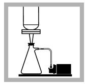
**9.** Connect vacuum to the filter holder/flask assembly again.
