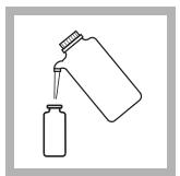
**3.** Fill a sample cell to the 10-mL mark with deionized water (the blank).
