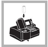
**4.** Place the blank into the cell holder. Close the light shield.
