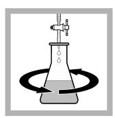
**8.** Put the flask under the buret. Swirl the flask. Add titrant until the color changes from yellow to redbrown.
