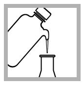
**5.** If the sample volume is less than 100 mL, dilute to approximately 100 mL with deionized water.
