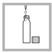
2. Pipet 2.0 mL sample into the digestion vial.
