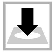
10. Insert the vial combination into the cell holder (blue indicator vial downwards). DR 1900: Go to LCK/TNTplus methods. Select the test, push READ.
