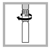
5. Immediately close the digestion vial tightly with the prepared indicator vial. Hold vial combination vertically. Do not invert.
