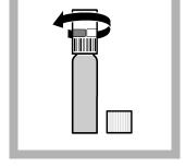
4. When the sample preparation is complete, open the blue indicator vial and immediately screw on the membrane double cap tightly. (The barcode label must point towards the indicator vial).
