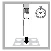
6. Heat in the reactor 2 hours at 100 °C (212 °F) (blue indicator vial upwards).
