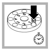
3. Insert the open digestion vial in the TOC-X5 shaker, pushing it down as far as possible. Position the fan cover over the vial. Switch on the instrument. After 5 minutes an acoustic signal is emitted.
