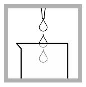
**3.** Use a pipet to add 1.0 mL of 10 N Sodium Hydroxide Solution to the sample.
