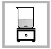
**2.** Add a stir bar and put the beaker on a magnetic stirrer. Stir at a moderate rate.
