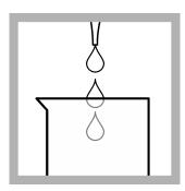
**10.** Add the standard solution to the beaker. Complete the remaining steps within 5 minutes.
