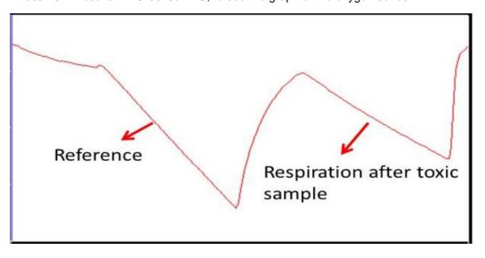
The reference measurement is the tracking of the oxygen consumption of the sludge with a suitable substrate.
