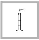
**5.** Add the contents of one Dechlorinating Reagent Powder Pillow to one cylinder. Stopper and invert several times until dissolved. This solution is the blank. The other solution is the prepared sample.
