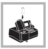
11. Place the prepared sample into the cell holder. Close the light shield. Results in mg/L ClO<sub>2</sub> (or chosen units) will be displayed.
