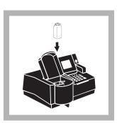
**9.** Place the blank into the cell holder. Close the light shield.
