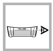
**4.** Fill the sample cup to the fill-line with sample.
