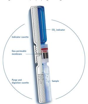
Figure 2:  $CO_2$  gas crosses the gas-permeable membrane into the indicator vial
