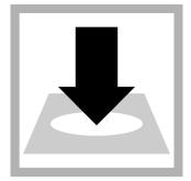
10. Insert the vial combination into the cell holder (blue indicator vial downwards).
