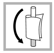
**9.** Invert the vial combination, thoroughly clean the outside of the **indicator vial** and evaluate.
