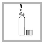
**2.** Pipet **1.0 mL sample** into the digestion vial.
