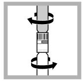
**8.** Tighten the vial combination **again** before inverting it.
