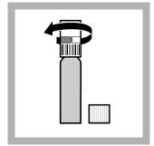
4. When the sample preparation is complete, open the blue indicator vial and immediately screw on the membrane double cap tightly. (The barcode label must point towards the indicator vial).
