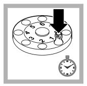
3. Insert the open digestion vial in the TOC-X5 shaker, pushing it down as far as possible. Position the fan cover over the vial. Switch on the instrument.
