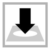
**5.** Insert the vial into the cell holder. DR 1900: Go to LCK/TNTplus methods. Select the test, push **READ**.
