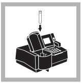
11. Place the sample in the adapter with the Hach logo facing the front of the instrument. Close the light shield.
