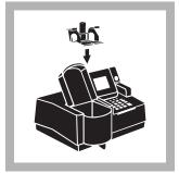
**3.** Insert the COD adapter into the sample module by sliding it under the thumbscrew and into the alignment grooves. Fasten with the thumbscrew.
