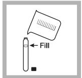
**4.** Fill an empty Test 'N Tube (TNT) vial with sample (the blank).
