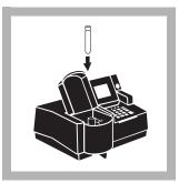
**6.** Place the blank into the adapter with the Hach logo facing the front of the instrument. Close the light shield.
