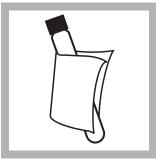
**10.** Within 30 seconds after mixing, wipe the vial containing the prepared sample.
